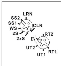
**With the top rotary switch** in the setting LRN up to 35 wireless pushbuttons can be assigned therefrom one or more central control pushbuttons. The required function of this multifunction impulse switch can then be selected. Switching will be visualised by flashing of the LED.
