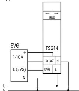
For the control from several LED drivers with 1-10V passive interface, an additional voltage source is necessary, this can be the power supply unit SNT12-230V/12V DC-0.5A or SNT61-230V/12V DC-0.5A, in both cases a 1kOhm resistor is necessary.
