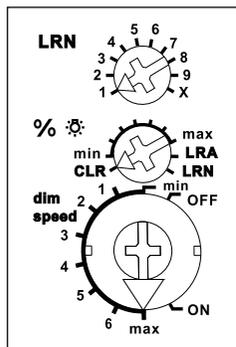
The minimum brightness (fully dimmed) is adjustable **with the % rotary switch**. The dimming speed is adjustable using the **dimming speed rotary switch**.
