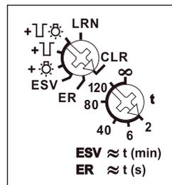
**With the top rotary switch** in the setting LRN up to 35 wireless pushbuttons can be assigned therefrom one or more central control pushbuttons. In addition wireless window/door contacts with the function N/O contact or N/C contact while the window is open. The required function of the impulse switch with integrated relay function can then be selected:
