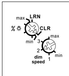
**The minimum brightness (fully dimmed) is adjustable with the % rotary switch.** In the setting LRN up to 35 wireless push-buttons can be assigned therefrom one or more central pushbuttons.
